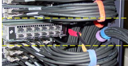
Figure 2-9 Removing a Leaf Card
