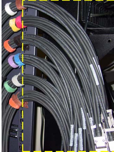
Figure 2-4 24-inch Cable Lengths
