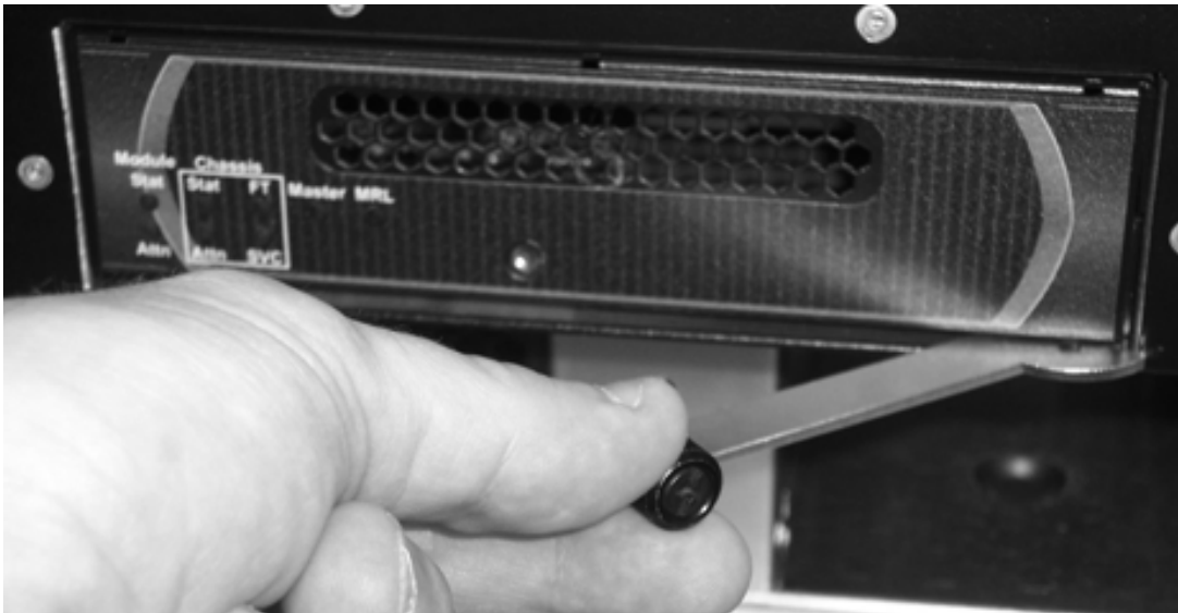
Figure E-12 12800 Management Module Removal
