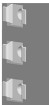
Figure 1-10. Clip Nut Orientation
