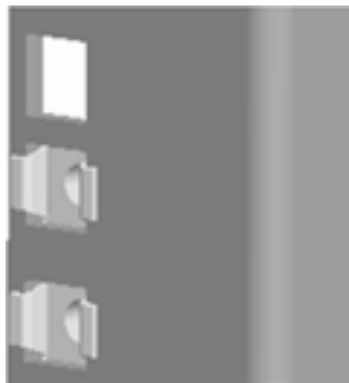
Figure 1-14. Clip Nut Orientation
