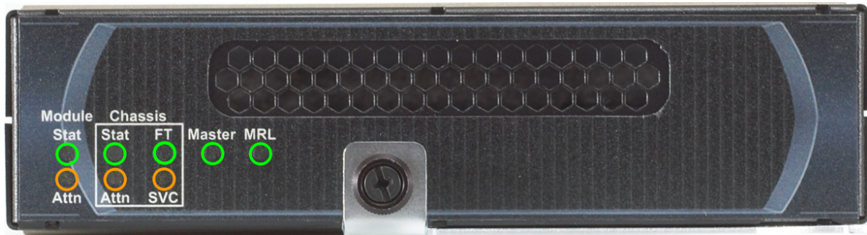
Figure 1-55. Management Module LEDs
