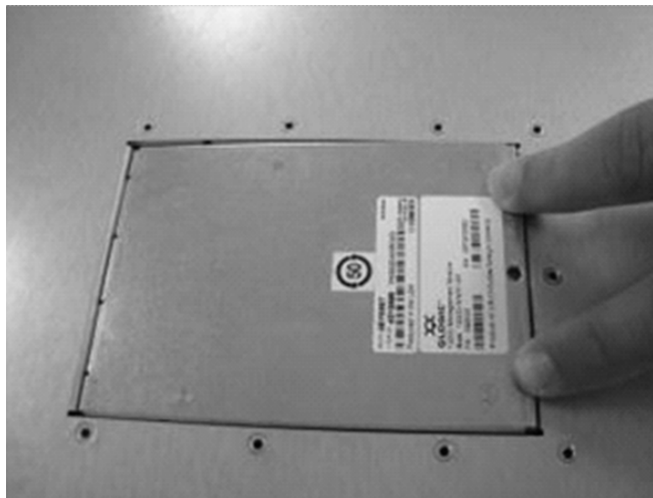
Figure E-3 12200 Management Card Insertion (2)
