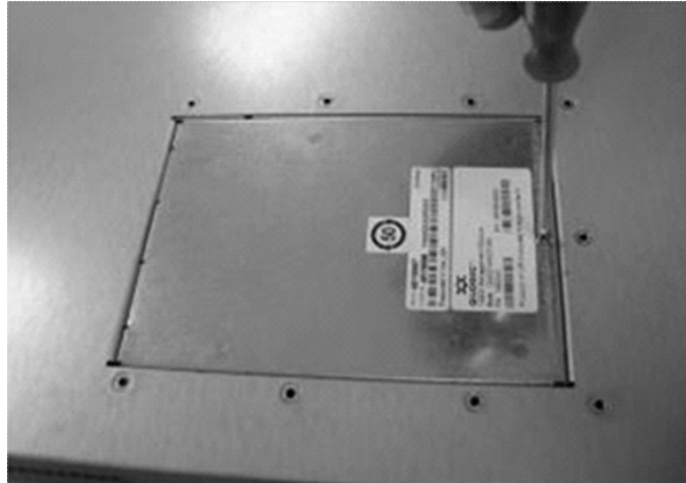
Figure E-4 12200 Management Card Insertion (3)
