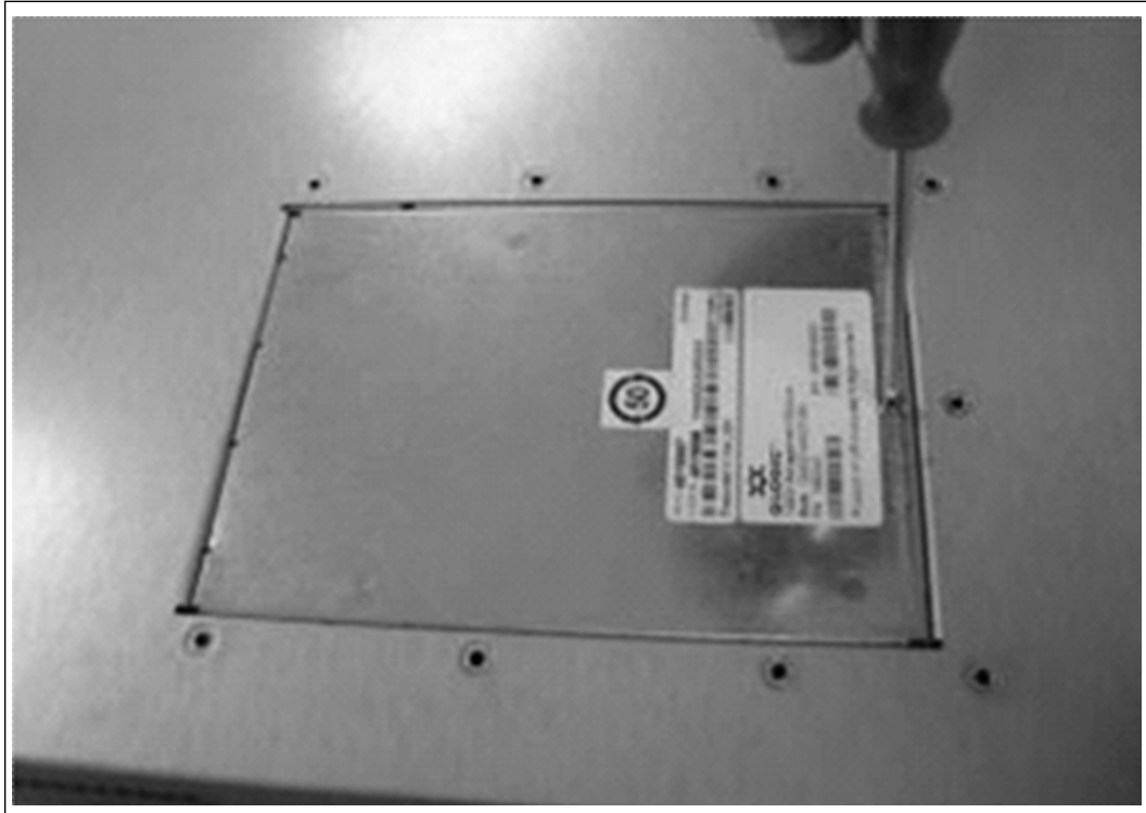
Figure 69. 12200 Management Card Insertion (3)
