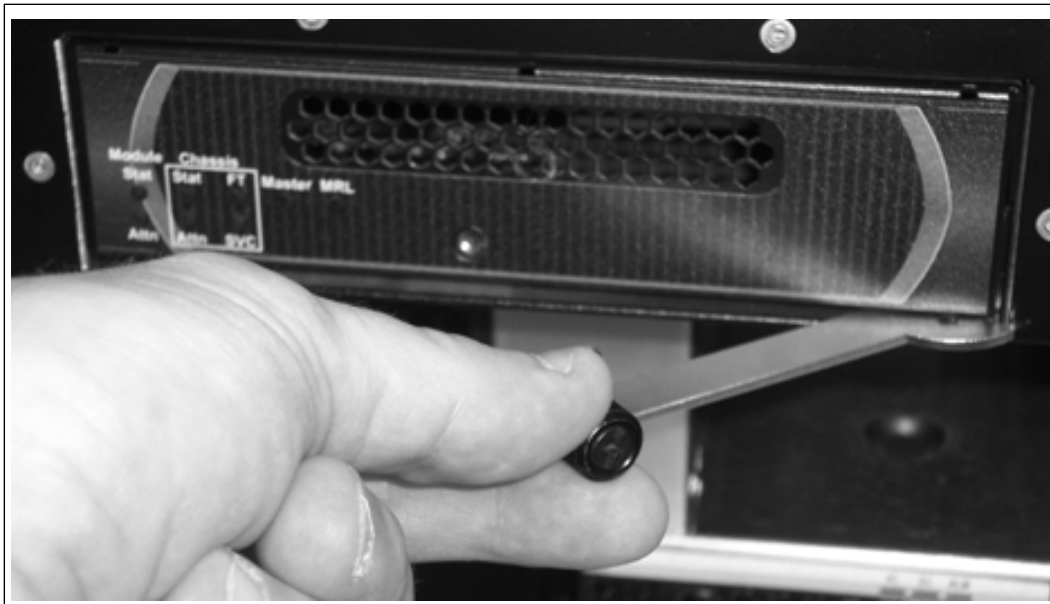
Figure 77. 12800 Management Module Removal
