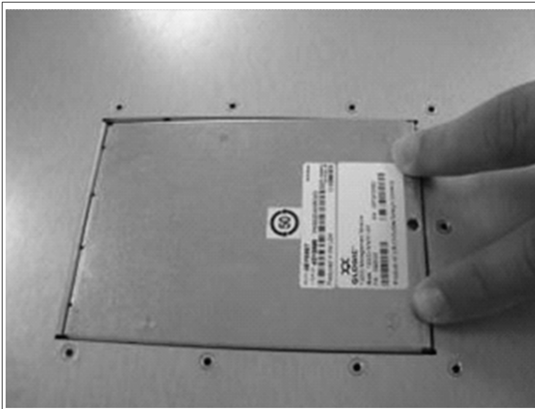
Figure 68. 12200 Management Card Insertion (2)
