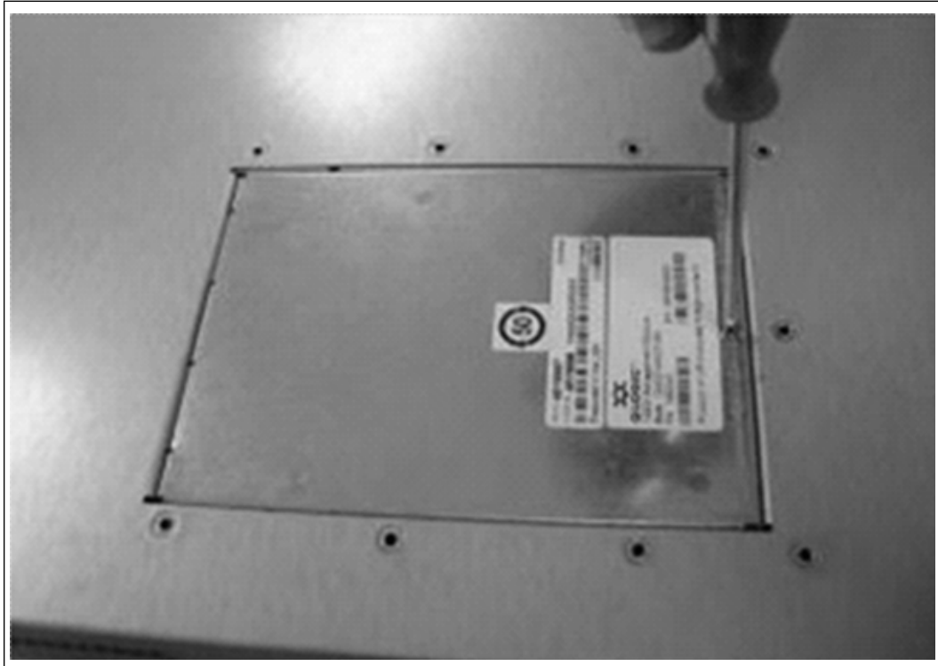
Figure 69. 12200 Management Card Insertion (3)
