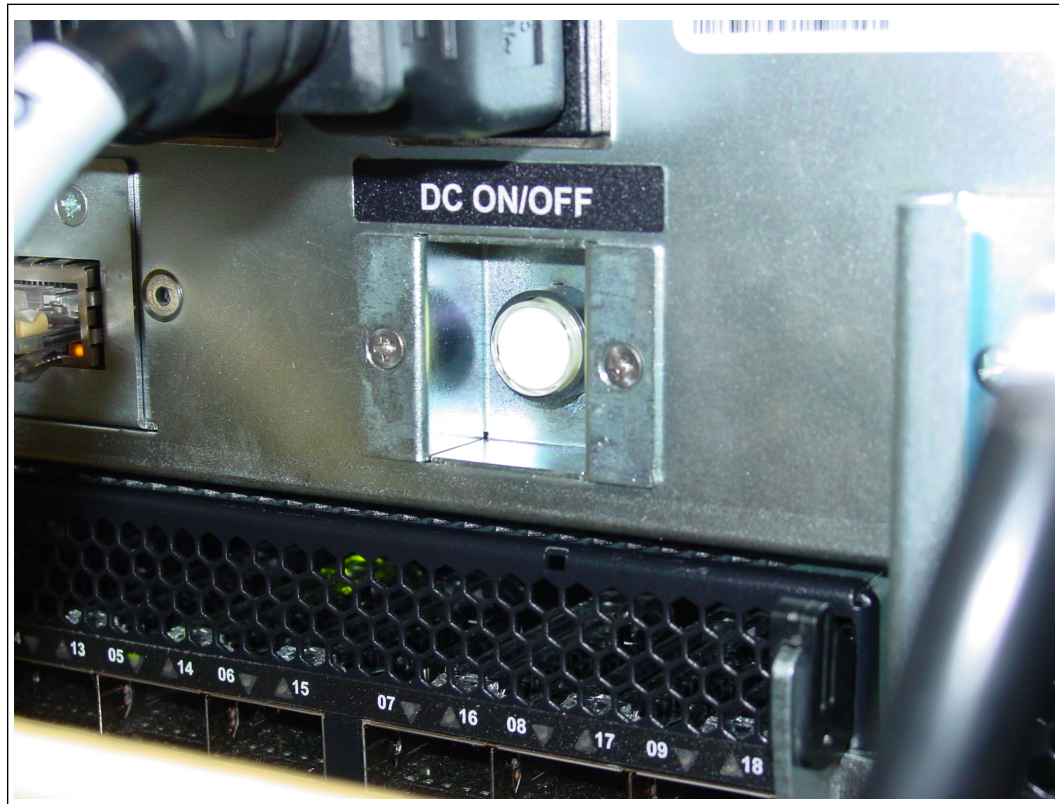
Figure 43. DC ON/OFF Switch
