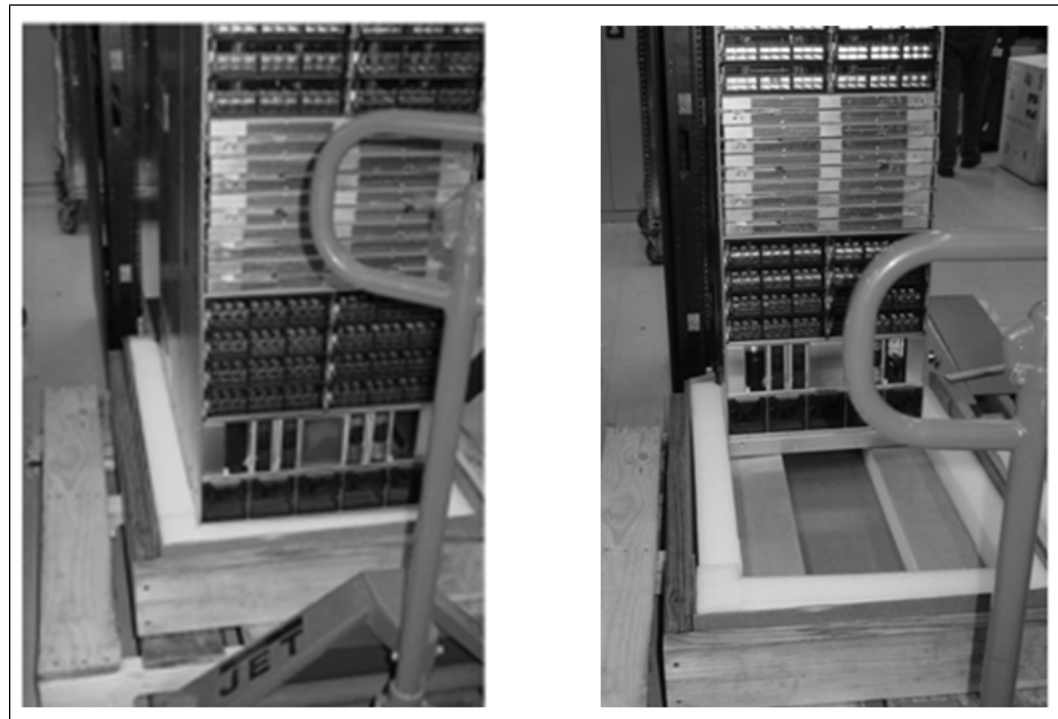
Figure 37. Sliding the Switch off the Pallet
