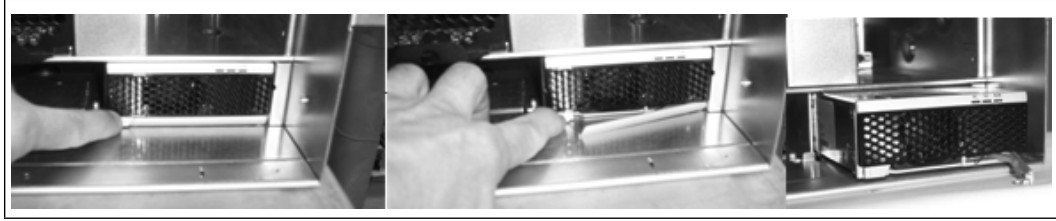
Figure 73. 12800 Power Removal
