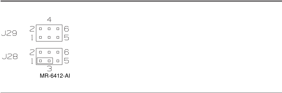
Figure 2–10 SROM Select Jumper Positions (J28 and J29)
