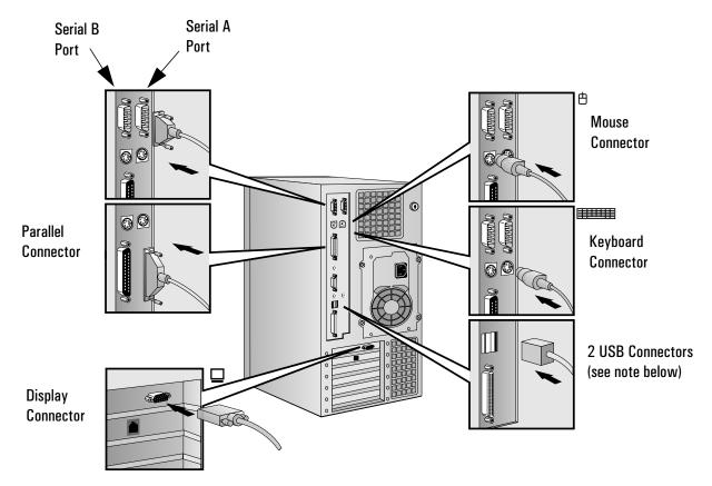
Connect the printer cable to the back of the computer and tighten the attachment screws. Use the connector labeled:
