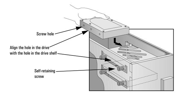
7 Secure the drive with the four self-retaining screws.
