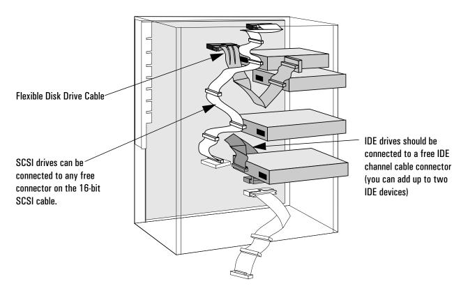
8 Connect the data and power cables to the rear of the device. (The connectors are shaped to go in one way only.)
