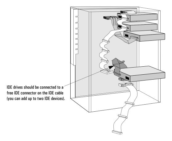
9 Connect the power cable and the data cable to the rear of the drive. (The connectors are shaped to go in one way only.)
