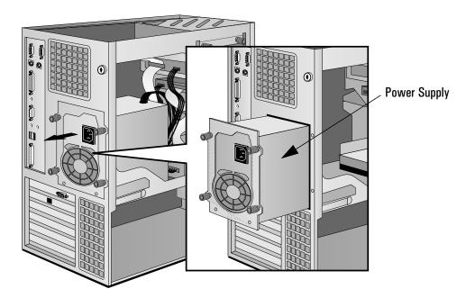
Slide the power supply unit clear of the computer
