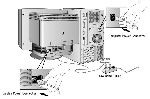
3 Connect the display's power cord and the computer's power cord to grounded outlets.
