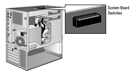
Switches 1 through 5 are used for processor settings (see page 52) and should not be changed. Replacing the processor with a different processor is not supported by HP.
