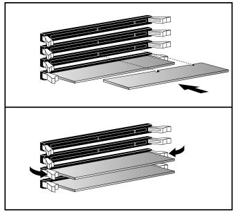
Slide the memory module into the slot at  $90^{\circ}$  to the system board
