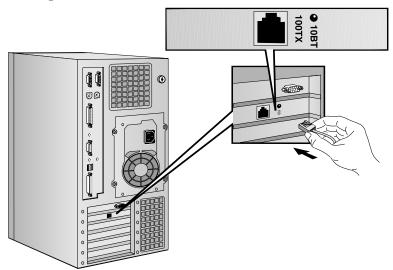
2 Attach the other end of the LAN cable to a hub (or into a wall socket that is connected to a hub).
