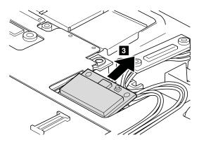
When installing: In models with the wireless USB adapter, plug the yellow cable into the jack on the card.
