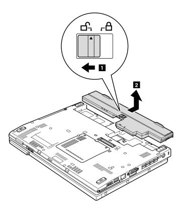
When installing: Install the battery pack along the slide rails of the slot. Then make sure that the battery release lever is in the locked position.
