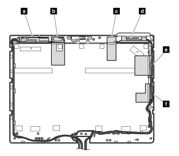
Attention: As you route the antenna cables, make sure that they are not subjected to any tension. Tension could cause the cables to be damaged by the cable guides, or a wire to be broken.
