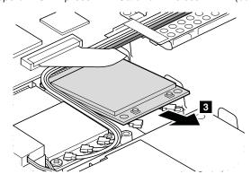
**When installing:** When you install the card, plug the red cable into the jack labeled **MAIN** on the card, and the blue cable into the jack labeled **AUX**.
