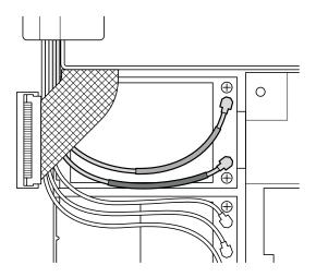
If the computer you are servicing is the wireless WAN-ready model, put the antenna cables in the cable protection tube and place them as shown in this figure.
