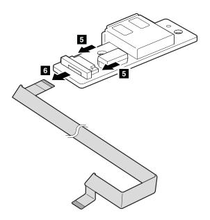
When installing: Route the cable as shown in this figure.
