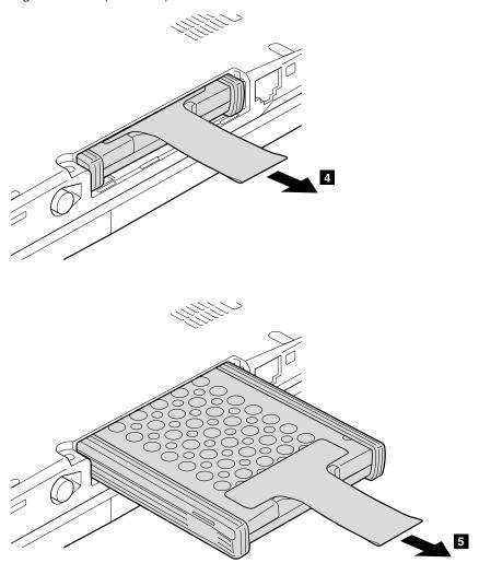
When installing: Make sure that the HDD connector or SSD connector is attached firmly.
