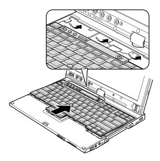
3. To make sure that the front side of the keyboard is housed firmly, gently press the keys with your thumbs and try to slide the keyboard toward you.
