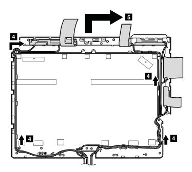
Table 39. Removal steps of LCD rear cover and wireless antenna cables (continued)
