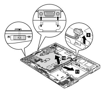
**When installing:** Make sure that the position of the wireless switch, and firmly fit into the frame **b**.
