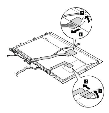
When installing: Make sure that the LCD cable connector are attached firmly.
