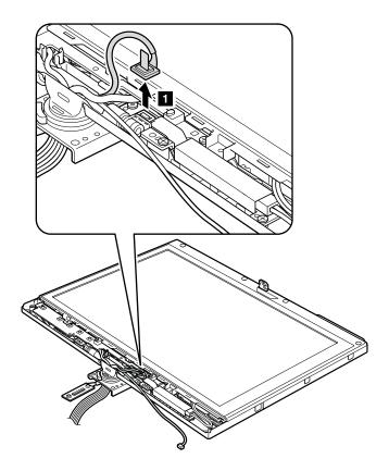
When installing: Make sure that the connector **1** is attached firmly.
