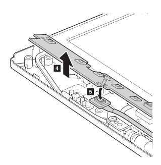
When installing: Make sure that the connector **5** is attached firmly.
