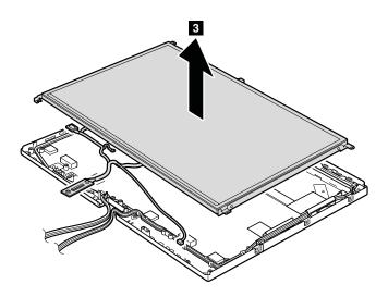
Table 37. Removal steps of LCD panel and LCD cable for Touch panel and Tablet Digitizer Pen model (continued)
