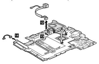
When installing: Make sure that the DC-in connector, the fan connector, and the Pen switch connector are attached to the system board firmly.
