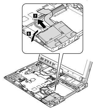
Turn the I/O card over, and then disconnect the cable from the flip-lock ZIF connector.
