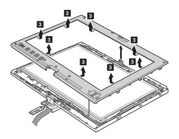
When installing: Make sure that all the claws are attached firmly.
