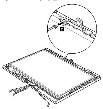
When installing: Make sure that the connector **2** is attached firmly.
