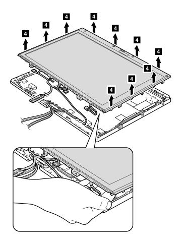
When installing: Make sure that all the claws are attached firmly.
