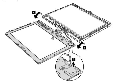
When installing: Make sure that attach the fingerprint reader connector firmly.
