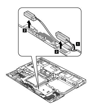
**When installing:** Route the speaker cables along the cable guides as shown in this figure.
