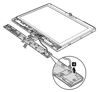
When installing: Attach the fingerprint reader connector firmly.
