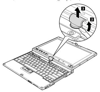
Table 15. Removal steps of hinge caps (continued) Close the LCD unit, and then remove the hinge cap (rear).
