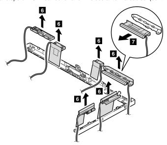
Remove the center latch from the LCD rear cover.
