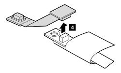
When installing: Make sure that the connector 4 is attached firmly.
