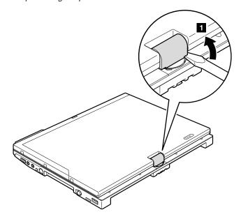
Open the LCD unit, and then remove the hinge cap (front).
