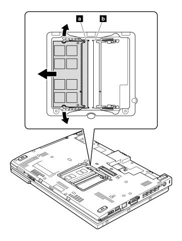
**When installing:** Insert the notched end of the DIMM into the socket. Press the DIMM firmly, and pivot it until it snaps into the place. Make sure that it is firmly fixed in the slot and does not move easily.
