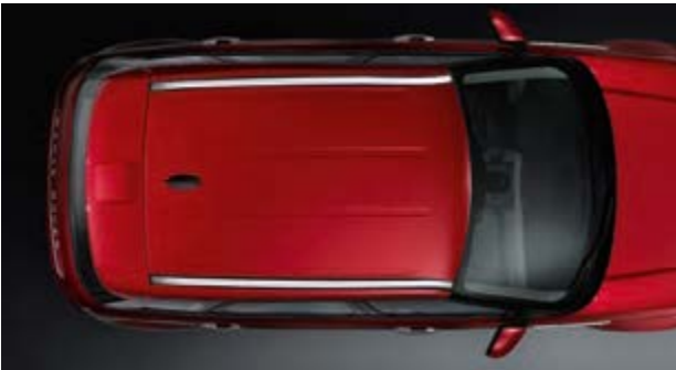
Roof Rails* Δ VPLVR0085 – Silver Finish VPLVR0086 – Black Finish Roof rails facilitate easy fitment of cross bars for roof carrying. Pre-set positioning points ensure cross bars are fixed in optimum position for weight distribution and dynamics. Vehicle height when fitted: Range Rover Evoque 1,640mm, Range Rover Evoque Coupé 1,609mm. Maximum permissible load capacity 71.8kg. Silver Roof Trim Finisher VPLVR0088 – Solid Roof
