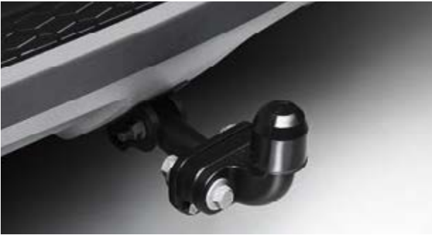
Towing System – Fixed Height Flanged Tow Bar VPLVT0170 Range Rover Evoque bolt-on flanged tow ball system with a 2,000kg load capacity (Convertible 1,500kg). A target tracking sticker is required for vehicles fitted with trailer assist option. 13 pin electrics is required for fitment (VPLHT0061).
