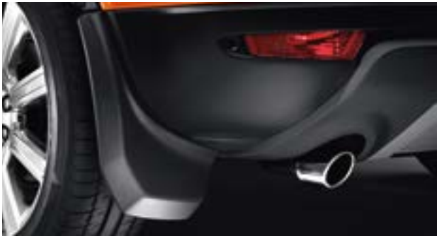
Rear Mudflaps** VPLVP0070 Mudflaps to reduce spray and help protect paintwork.
