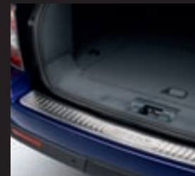
Stainless Steel Rear Bumper Tread Plate LR007321 Provides protection to the upper surface of the rear bumper. Compatible with all models except vehicles fitted with Stormer Accessories Pack, 2005-2009 Model Year.
