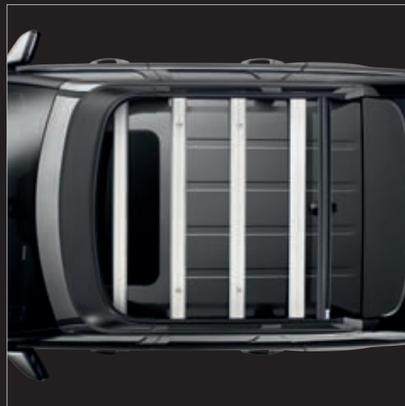
Roof Rails and Crossbars* VUB502130 Crossbars easily removed when not in use. Vehicle height when fitted 1,873mm at normal ride height. Load capacity 71.8kg.
