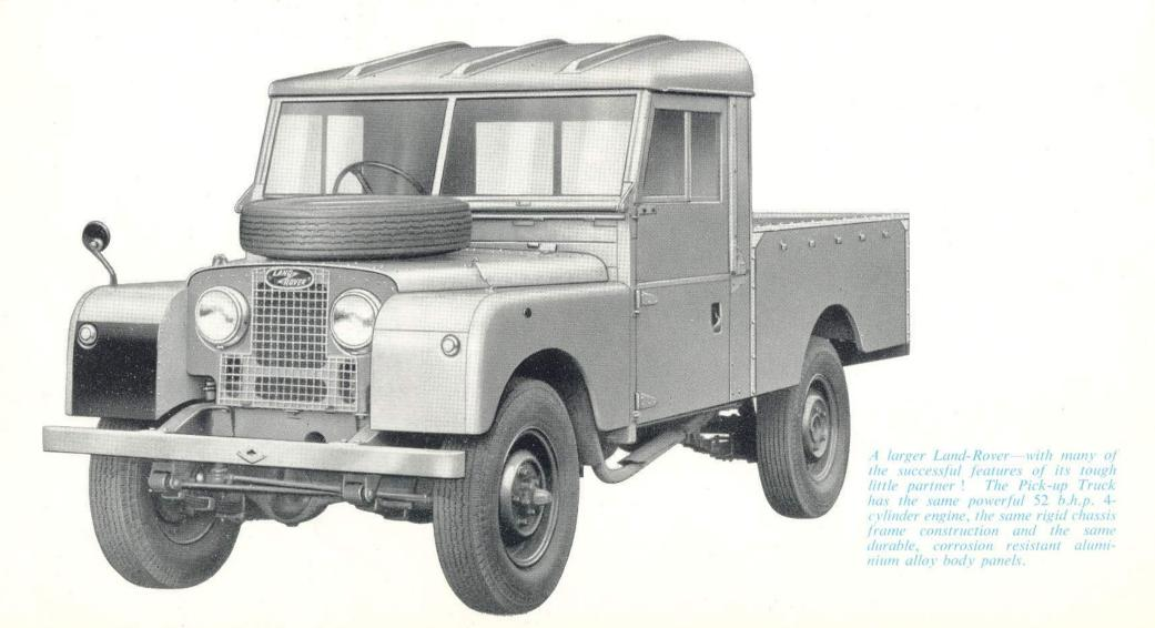
A 6-ft, long rear section provides ample load space for extra-bulky loads. There are handy lockers in the rear wheel-arches. A canvas hood to cover the rear section is available as an optional extra, also a tonneau cover.
