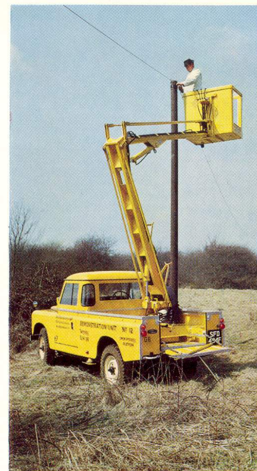
The vehicle provides an effective base on which to mount an hydraulically operated lift-platform. This type of equipment is in current use with many civic authorities for high-level maintenance tasks.
