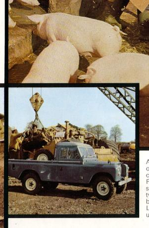
A 2.6 litre 1-ton Land-Rover is available for operators who require a greater load-carrying capacity (three persons plus 2240 lb). Features include heavy-duty axles and suspension, servo-assisted brakes, larger tyres and wider wheels, lower-ratio steering box, and a hydraulic steering damper. Low-speed performance is maintained by the use of lower transfer box ratios.
