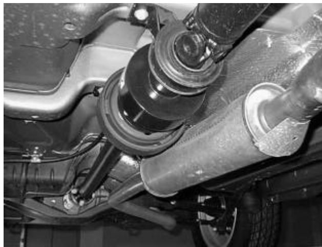
Rear of the front prop together with the VCU and bearings.
