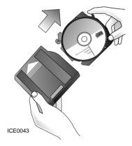
Holding the magazine as shown (arrow on magazine casing uppermost), remove each CD tray in turn.
