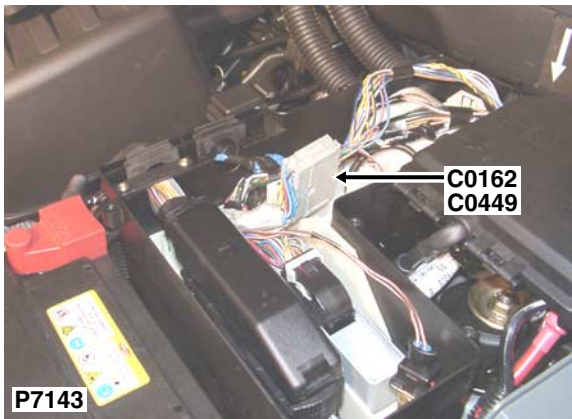
Description: Main harness to engine harness Location: Inside E-box
