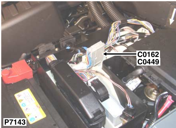
Description: Engine harness to main harness - KV6 Location: Inside E-box
