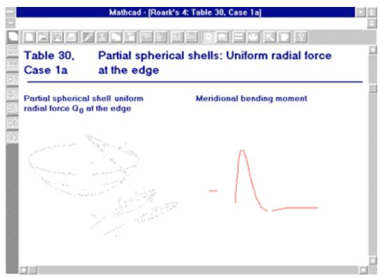
A "live" equation helps calculate uniform radial force on a partial spherical shell. The results can easily be seen in a graph.
