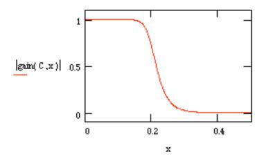
Finally we compute the gain for an FIR filter designed using the function bandpass.
