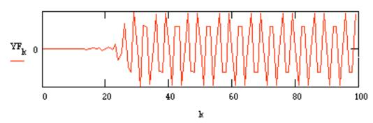
As a final example, we'll verify that the lowpass filter **G** defined above has 0 phase shift for several frequencies in the passband by plotting the filter output together with the input delayed by the filter delay of 18.
