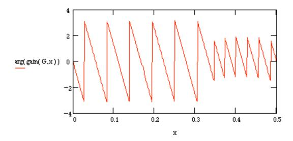
The phase is linear in the passband, as we'd expect, but we're seeing the effect of the filter delay. We can compute the complex gain relative to the delayed signal by dividing by the transfer function of the delay **D**, which is
