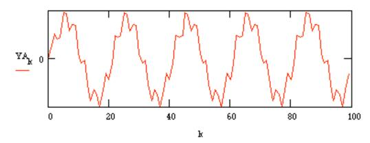
For the order 6 filter **C** the **response** function computes the response by feeding the output of the first section into the second section, and this output into the third:
