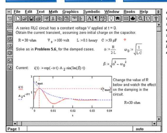
Given voltage resistance inductance and capacitance values, obtain the equation for the current transient. Then observe the effect varying resistance has on the damping of the circuit.
